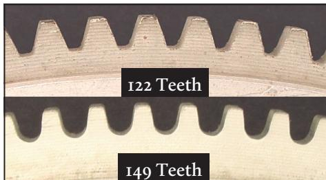
another useful general indicator, as the 122 tooth ring gear has V-shaped teeth, and the 149 tooth ring gear has U-shaped teeth (see photos at left). Close observation of the engine ring gear in question should suggest one of these two shapes, though heavy wear can obscure this visual indicator.
