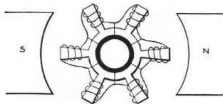
magnetic field. In the case of our SD-8, this magnetic field is provided by a series of permanent magnets that have been secured inside the perimeter of a cup-shaped housing. As this magnetic housing rotates around a fixed wire core, the result is alter-
