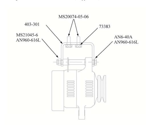
Step 3. Mount the 403-301-2 bracket to the engine case boss, using the two MS-20074-05-06 bolts and the 73383 locking plate. Torque the bolts to engine manufacturer's specifications or 110-150 in-lbs. Lock the bolts by bending the tabs on the locking plate up against the flats on the bolt hex.
