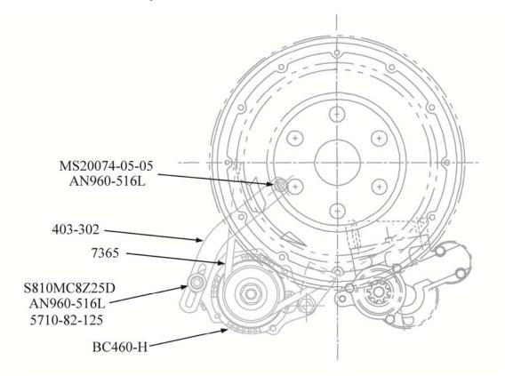
Step 5. Attach the 403-302 belt tension arm to the engine case using the MS-20074-05-05 bolt and an AN960-516L washer. Attach tension arm slotted end to alternator using the S810MC8Z25D bolt, an AN960-516L washer, and 5710-82-125 washer. Leave both bolts loose for belt adjustment.
