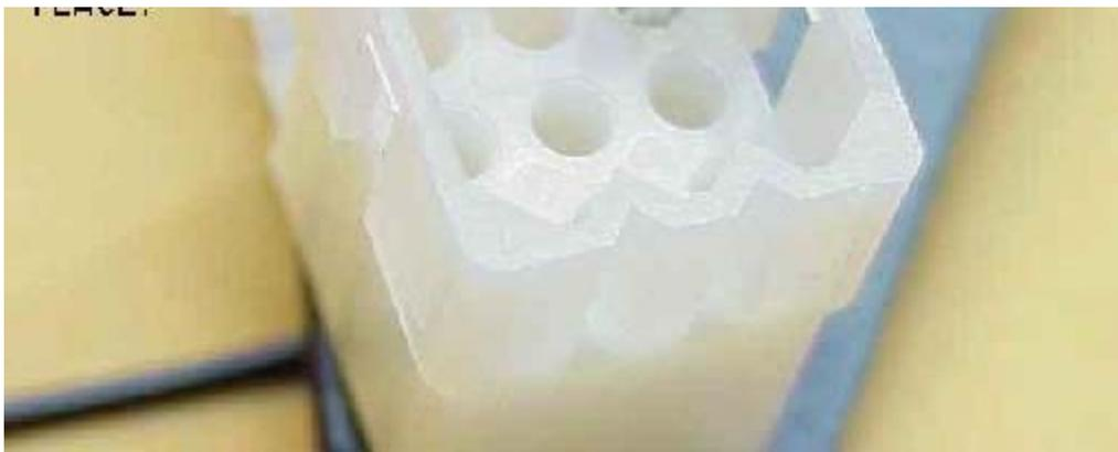
Wires of up to 14AWG and carrying up to 10 Amps may be routed through this style of connector. The wire I illustrated here is 20AWG. Use pocket "C" to crimp 16 and 14AWG wire. 22AWG wire is somewhat dicey in .093" pins. Waldom/Molex connectors also come in a smaller size having a nominal pin diameter of .063". Use pockets "E" and "B" to install the smaller pins like D-subminiature pins found on many instruments and avionics products.
