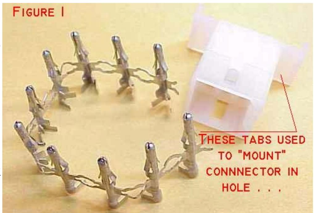
sized rectangular hole and hold the housing captive in the hole. Check the original manufacturer's data for recommended hole dimensions.
