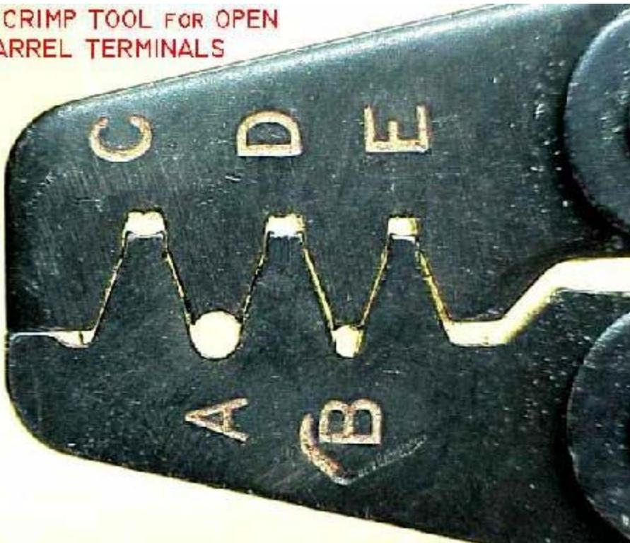
Closeup of the business end of our Open Barrel Terminal Crimp Tool. Note that pockets "C", "D" and "E" have "butt-cheeks" formed into the upper surface. These pockets cause the end of wire grip wings to curl over and dive into the approximate center of the wire strands. Pockets "A" and "B" have a smooth, circular shape used to shape the terminal's insulation-grips into a "bear hug" . . .
