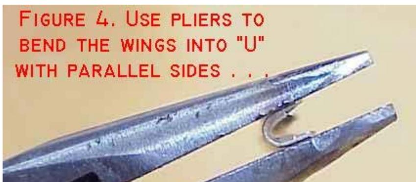
**FIGURE 4. USE PLIERS TO BEND THE WINGS INTO "U" WITH PARALLEL SIDES . . .**
