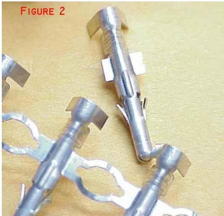
Pins supplied in strips are intended for application by automatic machine. The pins come in reels of perhaps 10,000 and feed into the side of an application machine like a chain of cartridges into a machine gun. For our use, we need to cut individual pins apart similar to what you see here. Note that part of the material that joins adjacent pins is left in place. It's too long in this view and will be snipped off again later.
