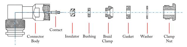
This connector is intended for use with a high-quality shielded coaxial cable, such as RG400:
