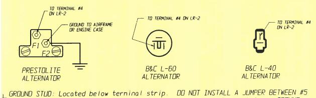
TUD: Located below terminal strip. DO NOT INSTALL A JUMPER BETWEEN #5
