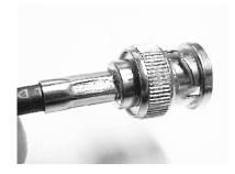
(5) Use .213" hex die in tool to put crimp over portion of ferrule that will capture braid wires against tailpiece of connector. Round end of die facing toward the coax cable. After crimping, trim free ends of braid with a knife.
