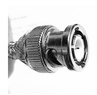
(4) Slide ferrule up on exposed shield braid until end of ferrule compresses ends of braid tightly against the back of the connector body.
