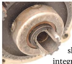
“lip seal” desiccates, and wears from normal pinion travel on its supporting shaft. Inevitably, as the integrity of this seal declines, engine oil migrates into—and through—the starter. Cracked pinions are another common problem for this starter design. With only 1/8” (approx.) of base material at its thinnest point, the pinion on these units is susceptible to fracture in cases of incomplete engagement at start-up, or as a result of severe engine kick-back.
