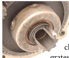
pinion travel on its supporting shaft. Inevitably, as the integrity of this seal declines, engine oil migrates into—and through—the starter. Cracked pinions are another common problem for this starter design. With only 1/8" (approx.) of base material at its thinnest point, the pinion on these units is susceptible to fracture in cases of incomplete engagement at start-up, or as a result of severe engine kick-back.
